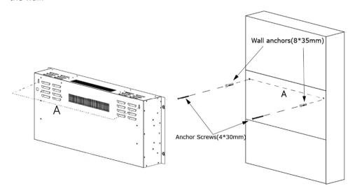
Step 3. Hang the fireplace on the wall and lock the T-shaped bracket
