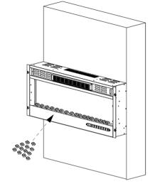
Step 5.Reinstall the glass panel and reinstall the screws.
