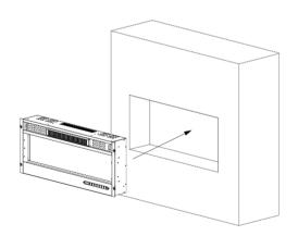
Step 3. Secure the fireplace Mark the left and right anchor screws secure positions on the wall in accordance with the fireplace s holes.
