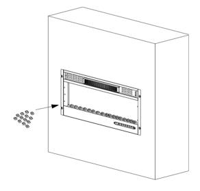
Step 5. Reinstall the glass panel Place the front glass panel over the front of the fireplace aligning the slots at each side of the glass panel with the lugs on the sides of the fire.
